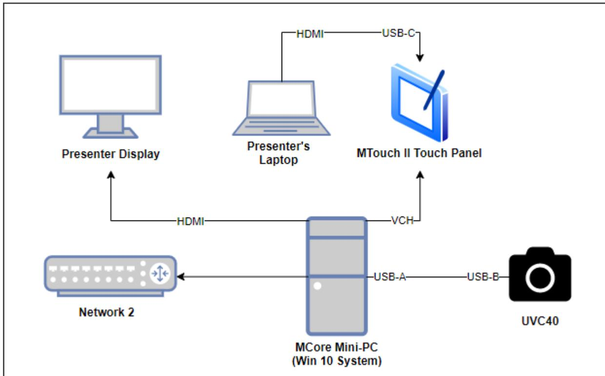
The test network topology above was used for the MVC400 deployment. With the MCore Mini-PC as the centerpiece, we connected it to the network and also connected to the Presenter's Laptop to the MTouch II Touch Panel.. This will act as the interface for the user. The Presenter's Display will show what the user decides based on their interactions with the MTouch II Touch Panel. The UVC40 will be the all-in-one camera, microphone, and speaker.
