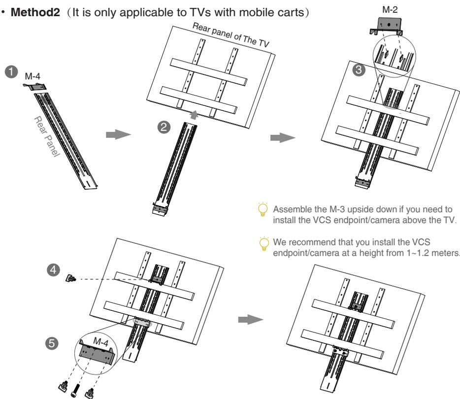
💡 Assemble the M-3 upside down if you need to install the VCS endpoint/camera above the TV.
