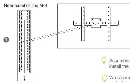
💡 Assemble the M-3 upside down if you need to install the VCS endpoint/camera above the TV.
