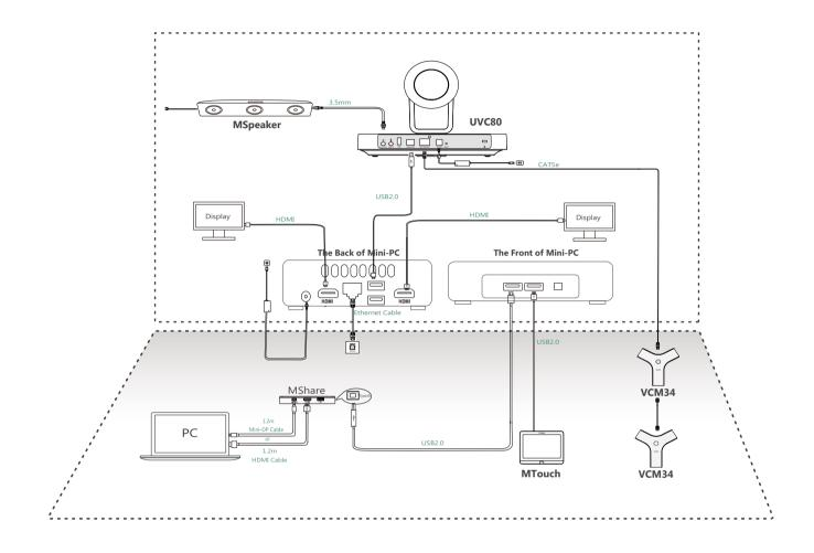
For convenience, we recommend that you connect a wireless USB dongle to the back of the Mini-PC to use mouse and keyboard to manage devices.
