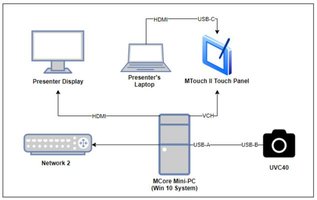
The test network topology above was used for the MVC400 deployment. With the MCore Mini-PC as the centerpiece, we connected it to the network and also connected to the Presenter's Laptop to the MTouch II Touch Panel.. This will act as the interface for the user. The Presenter's Display will show what the user decides based on their interactions with the MTouch II Touch Panel. The UVC40 will be the all-in-one camera, microphone, and speaker.
